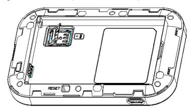
5. Place the SIM card gently with gold IC chip facing downward. Use the SIM picture engraved on device to make sure it is placed properly.
