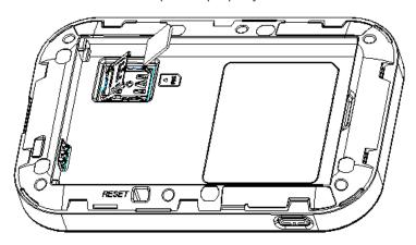
6. Flip the metal rectangular cover back on as shown below and while gently pressing the metal cover, slide towards the SIM picture to secure the SIM. (You will feel it lock.)
