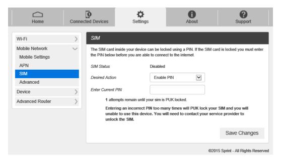
■ Enter the SIM PIN and press "Save Changes". The SIM Status will be changed to Enabled. Once the SIM PIN Lock is enabled, you need to enter the SIM PIN to connect to the mobile broadband network each time you power on your R910.
